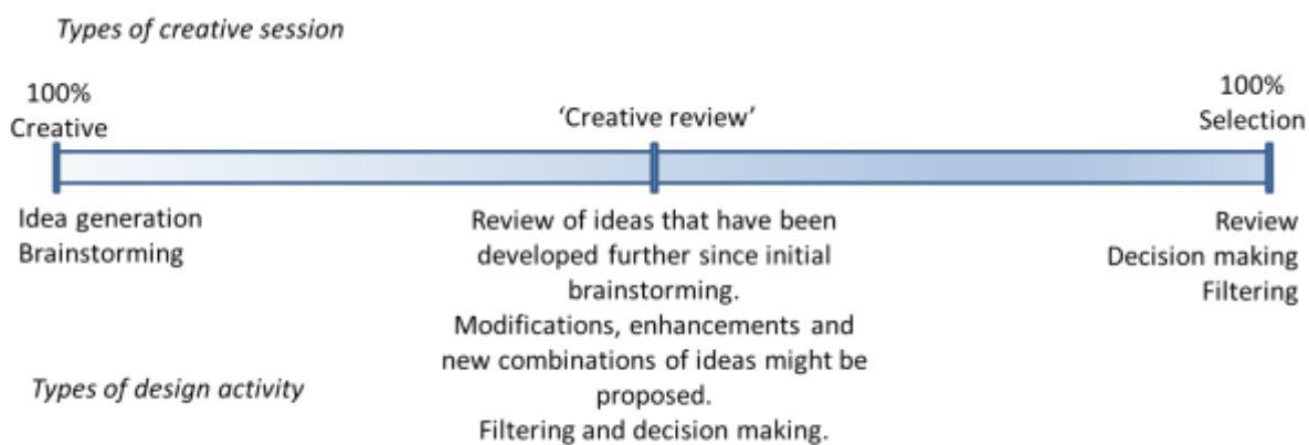
Figure 14. Types of creative session and design activity that could be supported by the SPARK platform.
